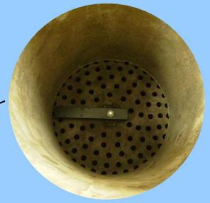
*Reactor with casted boiler grade refractory
