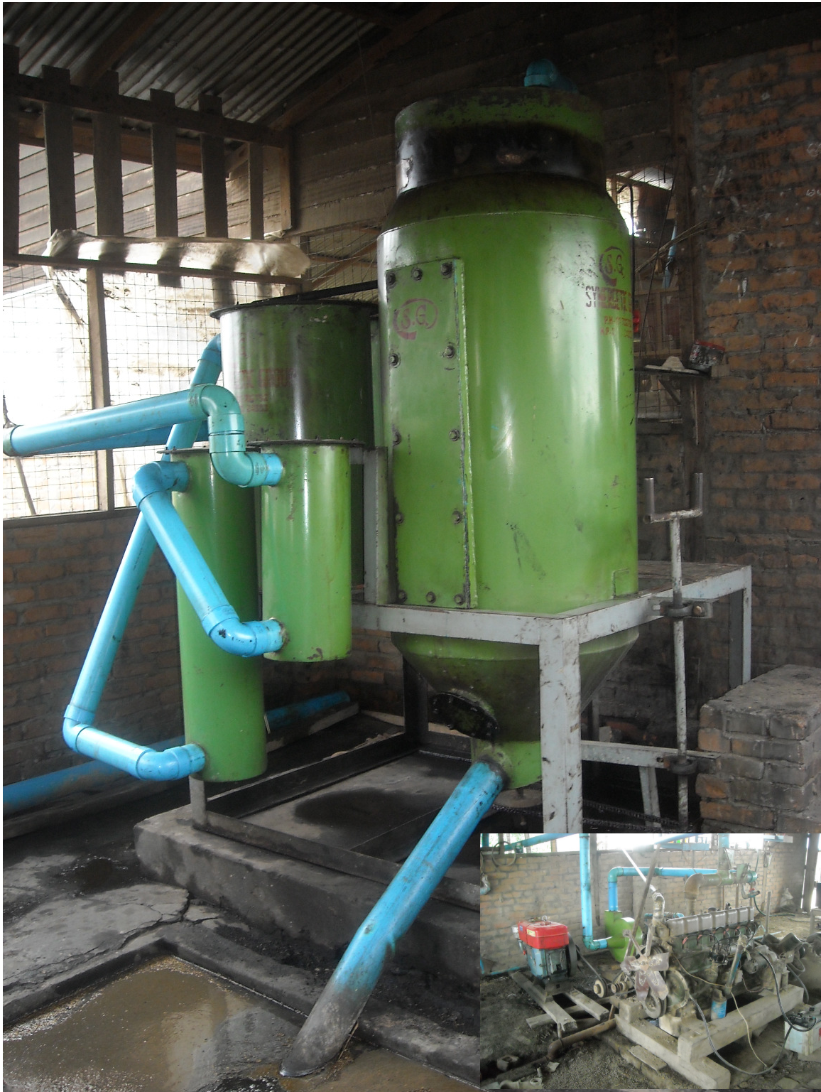
Fig 4. Model TG 180 powering a 105 horsepowers FAW gas engine (insert) operating in a rice mill in Azauk, Myanmar using rice husk. The TG 180 and the gas engine is the only power source for the rice mill since 2006.
